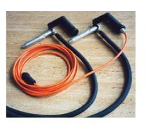
Mobile AC and HW current generator **MAGMAN 6000 H** is designed to generating of magnetic fields for magnetic particle testing according ASME Code V. 7, EN 1290, EN ISO 9934, ASTM A 275, ASTM E 709, ASTM E 1444 to testing of iron castings, forgings, welds and wrought parts. Outer switches can be switch in the handle of prod, footswitch or button from stationary bench.
