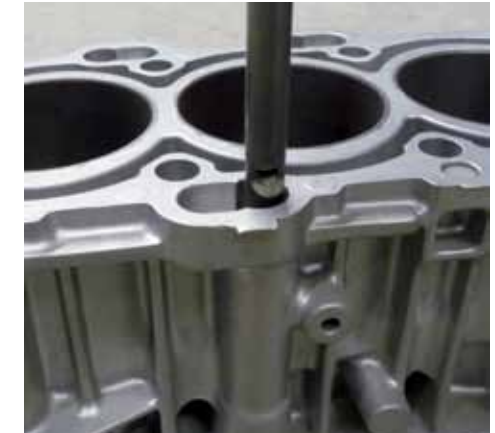
Inside blasting of crankcases
