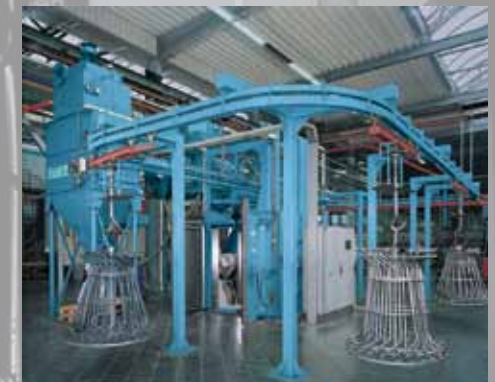
Transport of workpieces on monorail
