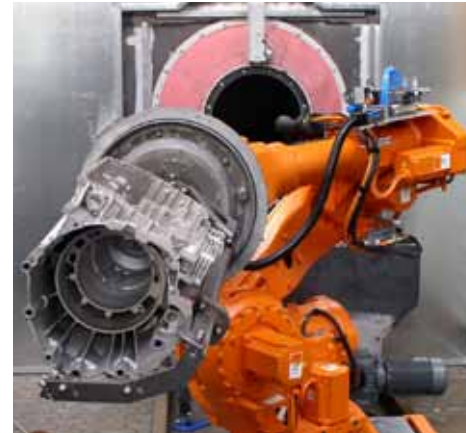
Finishing cell with Robot Gripper
