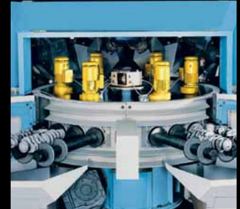
Fully automatic shot peening of more than 600 crank shafts / h on DS machine
