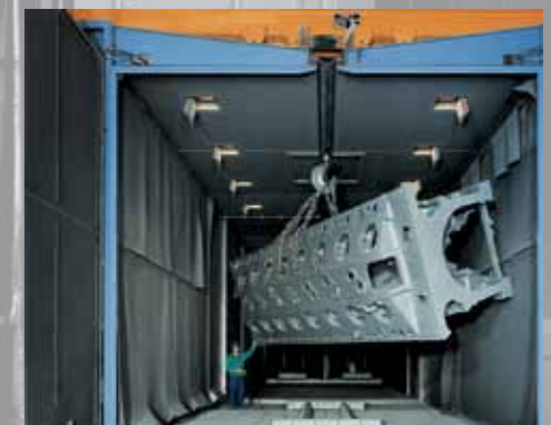
Blast house for a 80 tonne diesel engine block
