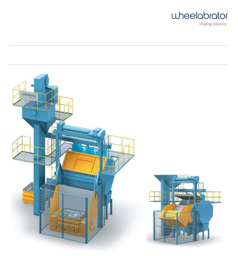
DTC blast cleaning machines are especially suitable for cleaning, decoring or descaling of tumbleproof work-pieces (forgings, castings). The polygon shaped drum ensures complete turning of the work-pieces for an optimal exposure of all surfaces to the blast stream. The intensity with which the parts are turned for thorough shot removal is the same as for blasting. The arrangement of the blast wheels ensures optimum blast cleaning and maximum utilisation of the abrasive energy.
