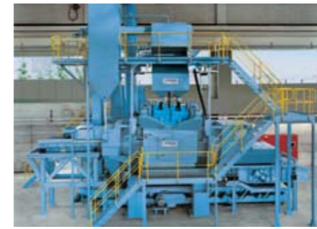
Blast cleaning machine with inlet and outlet vibratory conveyors
