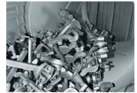
Parts in the outlet barrel after cleaning
