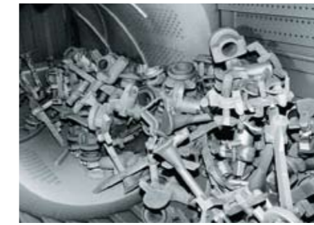
Uncleaned castings in the inlet barrel
