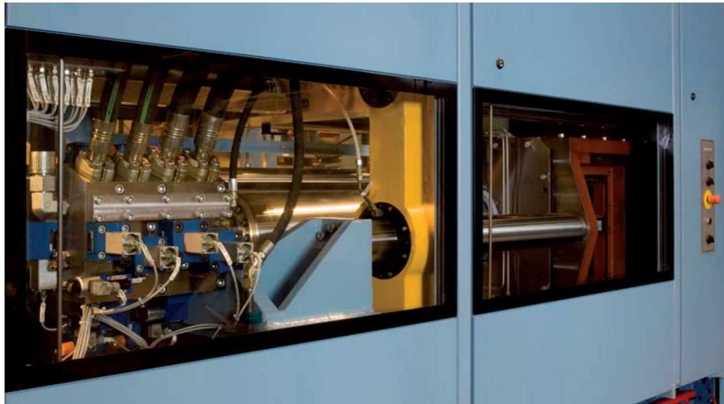
DISA 231 with inspection windows for easy surveillance
