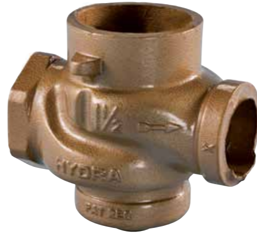
Flush Valve, 1.2 kg 4 per mould - DISAMATIC 2110 MK2
