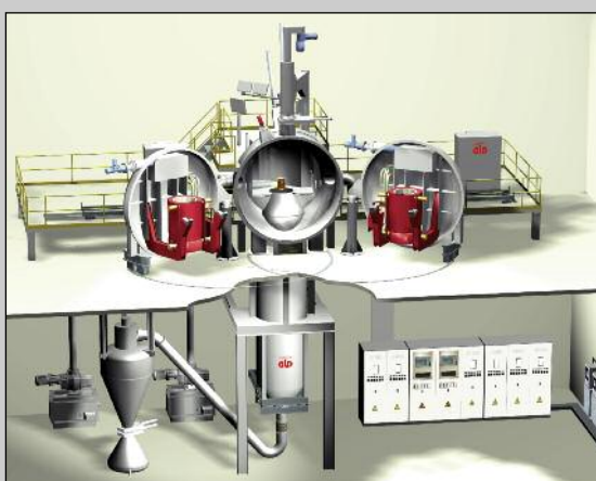
Schematic design of a large scale atomization unit with a double-door melting furnace chamber
