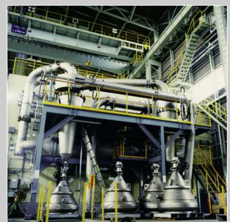
Powder collection system of a large-scale atomization unit
