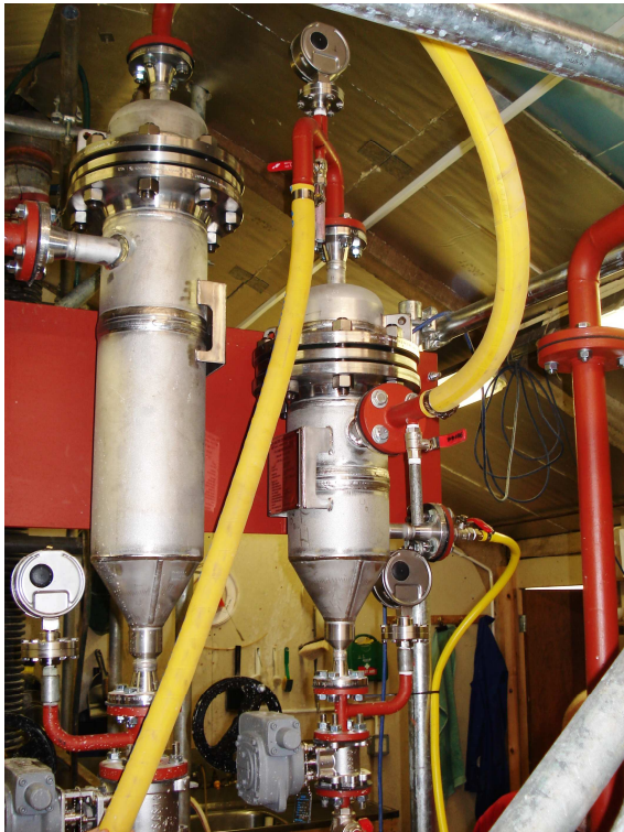
3 inch and 1 inch hydrocyclone pressure vessels under test at Salter Cyclones
